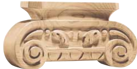
CPL-IP3 Capital Ionic Pilaster Large 9 3/4" w x 4 3/4" h x 2 1/2" thick Inside height: 4 1/4" Use with 5" column
